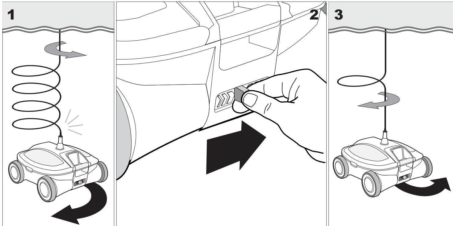
**EN****Setting up the axle lock lever for cable detangling**
