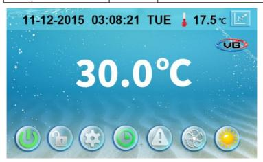
When the timerwas starting, the clock button is green in the main interface
