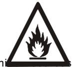
The appliance shall be stored in a room without continuously operating ignition
